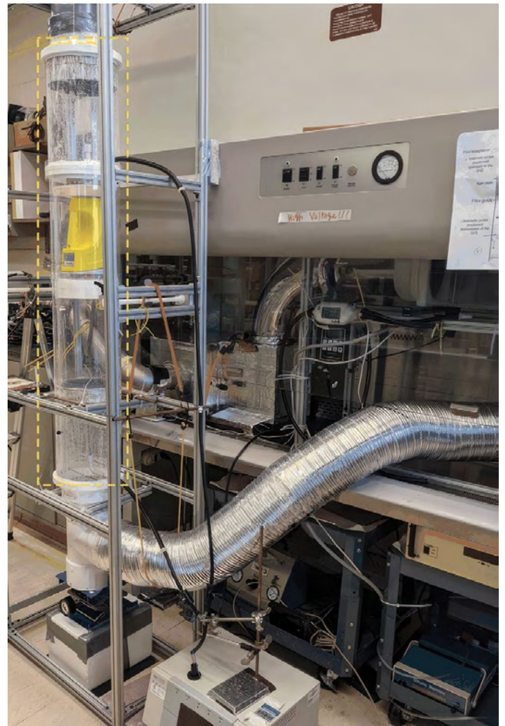
FIGURE 1: All presented air sampler configurations show a result of d_{50} < 2\mu m , so they are compliant with EN 17141 requirements.
