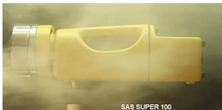
FIGURE 1: Average smoke deviation confirms that the airflow deviation is minimal, with no impacts on cleanroom applications.
