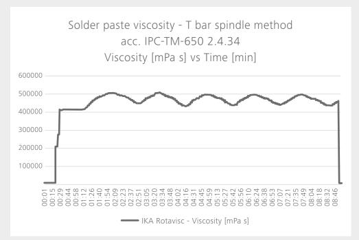
Note: The above data is obtained by the analysis of 5 cycles measurements recorded by IKA labworldsoft<sup>®</sup> 6 Visc. (Helistand up and down is one cycle)
